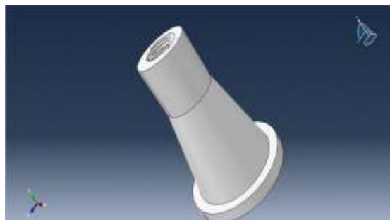
Fig 3: modeling of screw jack frame for square thread
