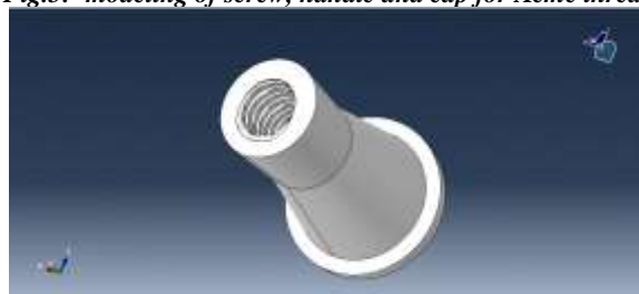
Fig.6:- modeling of screw jack frame for Acme thread
